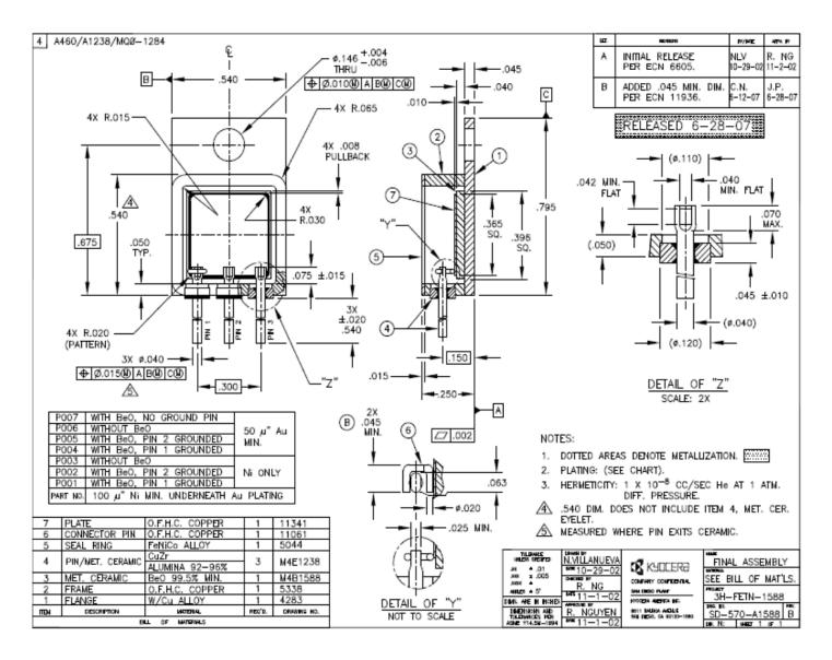
Pin Assignments: 1=Drain, 2=Source, 3= Gate
