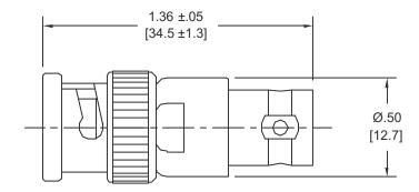
Note: Dimensions in Brackets are Expressed in Millimeters and are for Reference Only. Units that operate over a more specific frequency band and/or offer very low return loss (VSWR) are also available.
