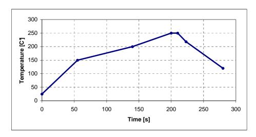
Tolerance for Temperature settings T +0℃ (according to JEDEC J-STD-020C, July 2004)
