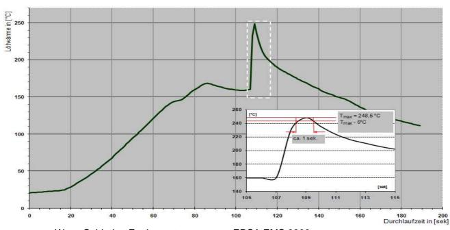
Wave Soldering Equipment: Throughput speed: 1m / min ERSA EMS 3300
