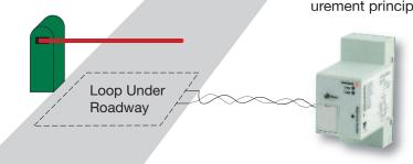
way and connected to the loop detector. The change in inductance when a vehicle is present will be measured as a change in frequency. The output relay operates when the loop is activated and releases again when the loop returns to non-activated condition. The loop detector is typi-
