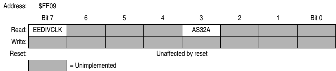
Figure 10-2. Mask Option Register 2 (MORB)
