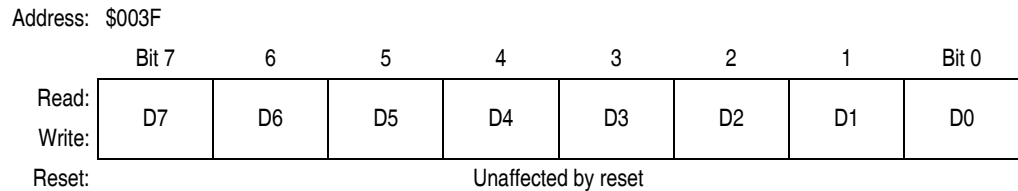
Figure 4-22. BDLC Data Register (BDR)
