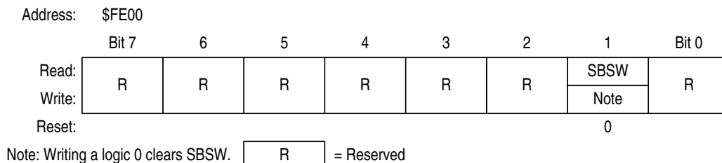
Figure 18-6. SIM Break Status Register (SBSR)
