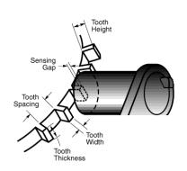
For best results we recommend targets made from low carbon cold rolled steel. Other factors that influence sensor performance include geartooth height and width, space between teeth, shape of the teeth and thickness of the target. As a general guideline consider a target with the following minimum parameters
