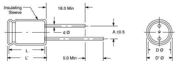
$D' \ Ø = D \ Ø + 0.5$  Max       $L' = L + 1.0$  Max at  $D \ Ø \leq 8.0$        $L' = L + 2.0$  Max at  $D \ Ø \geq 10.0$
