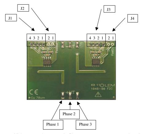
The board comprises two Minisens transducers, one for Phase 1 measurement, a second one for Phase 3; the Phase 2 in the centre is not measured.
