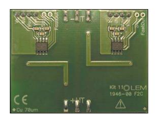
This evaluation board is based on a multi-turn design making possible a 2 phases measurement in a 3 phases system.
