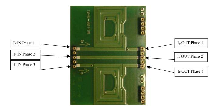
Connect then the primary phases according to the above picture, the positive direction being from  $I_P$  IN to  $I_P$  OUT.
