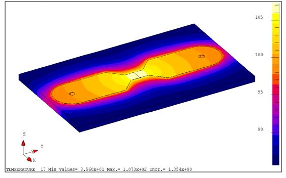
Track thickness 35  $\mu$ m, PCB thickness 1.6 mm,  $T_A$  = 85 °C, natural convection,  $I_{PN}$  = 10 A rms or A DC.
