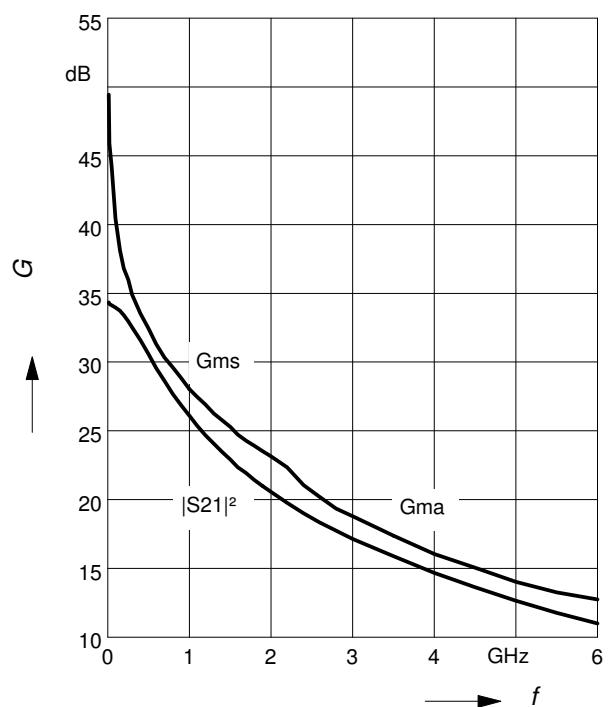
**Power gain**  $G_{\text{ma}}, G_{\text{ms}} = f(V_{\text{CE}})$
