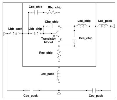
0.212 nΑ  $L_{\text{bb\_chip}} =$ 0.07472  $L_{\rm cc\ chip} =$ nΗ 0.0184 nΗ L<sub>bb</sub> pack = nΗ 0.277  $L_{\rm cc}$  pack = nΗ 0.239 L<sub>ee pack</sub> = 0.015 рF  $C_{\rm bc\ chip} =$ 0.013 pF  $C_{\text{cb\_chip}} =$ 0.282  $C_{\text{ce chip}} =$ рF 0.064 рF  $C_{\text{be pack}} =$ 0.0492 pF Cce pack = 7 Ω  $R_{\rm bc\ chip} =$ 0.566 Ω  $R_{\text{ee chip}} =$ Valid up to 6GHz
