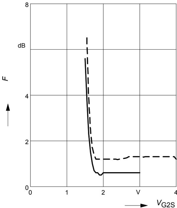
**Noise figure  $F = f(V_{G2S})$ ,  $f = 800\text{ MHz}$**
