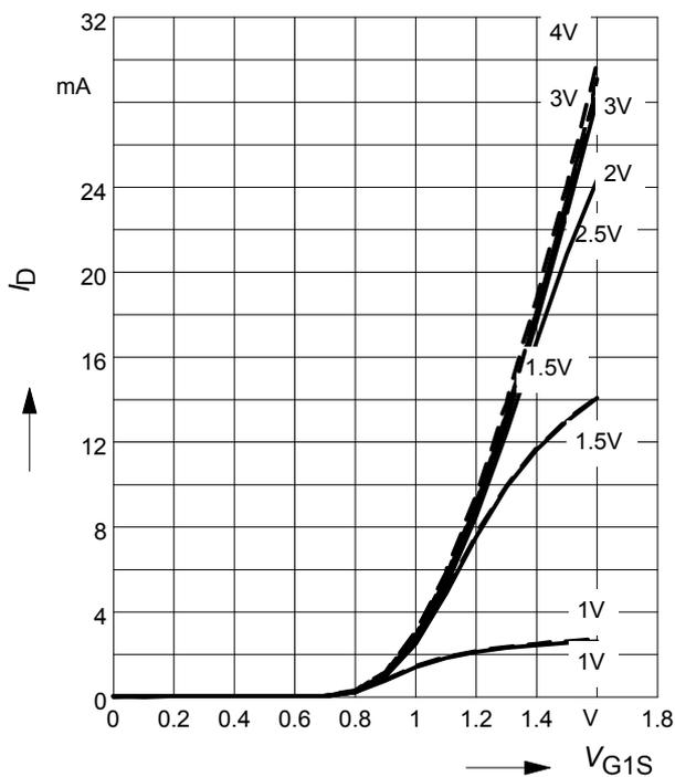
**Drain current  $I_D = f(V_{GG})$**
