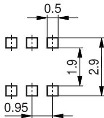
Remark: Wave soldering possible dep. on customers process conditions
