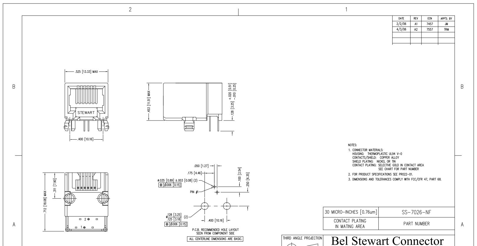
11118 Susquehanna Trail South Glen Rock, PA 17327—9199 (717) 235—7512 Fax: (717) 235—7954 http://www.stewartconnector.com DO NOT SCALE DRAWING TWO CONTACT, SIX POSITION, MICRO JACK, NON-FLANGE DRAWING IS SUBJECT TO CHANGE WITHOUT NOTICE DIMENSIONS: INCHES [METRIC] UNLESS OTHERWISE SPECIFIED TOLERANCES ARE ±.005 [0.13]
