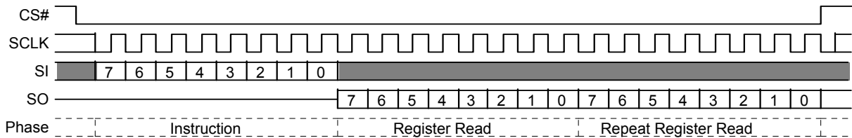
Figure 10.6 Read Configuration Register (RDCR) Command Sequence
