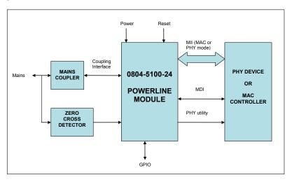
The block diagram presents the 0804-5000-24 powerline module in a typical environment. Eight different types of interfaces are observed. These interfaces are described in details below.
