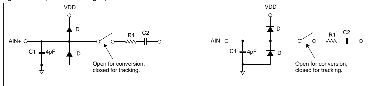
Figure 35. Equivalent Analog Input Circuit
