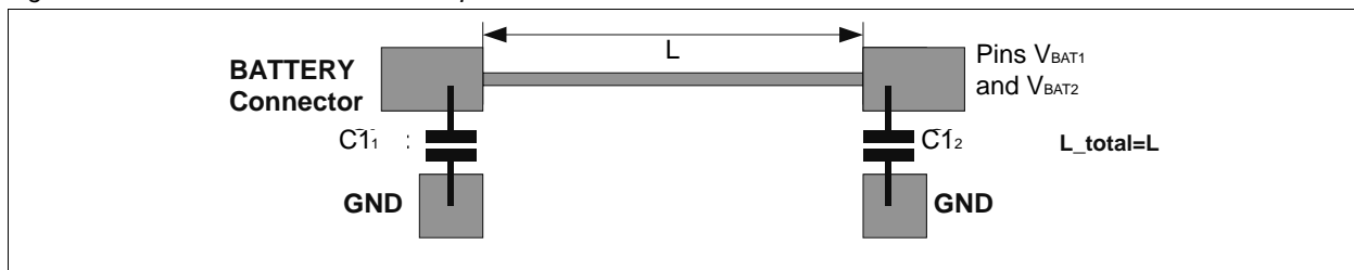
Figure 21. PCB Wire Inductance Example 2
