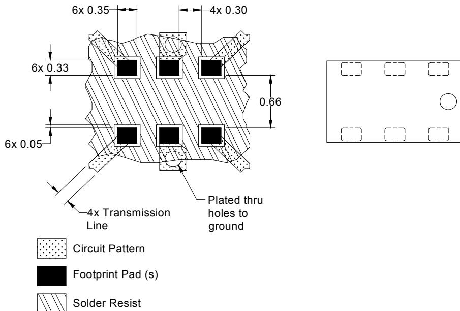
Dimensions are in Millimeters
