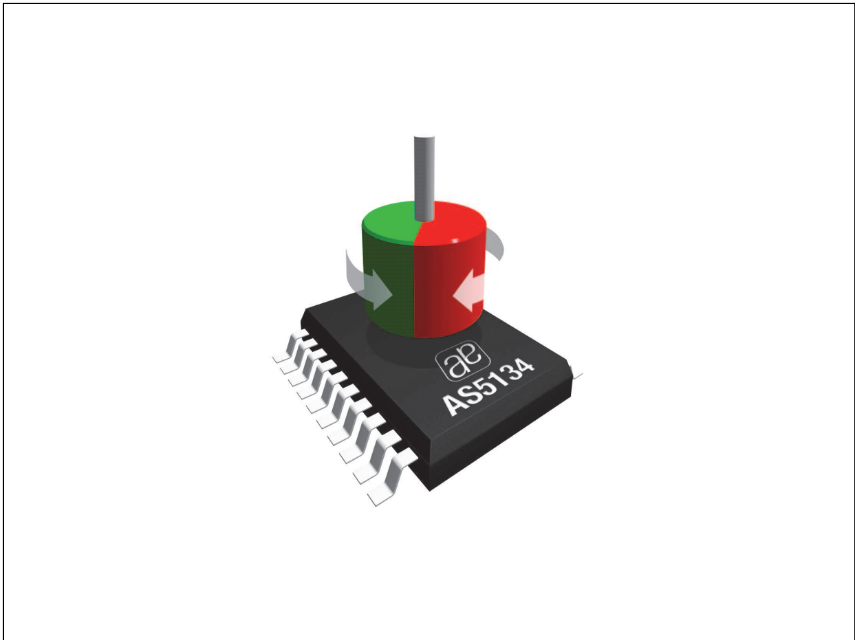
Figure 3. Typical Arrangement of AS5134 and Magnet
