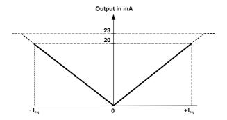
Note: 1) The performance specified in the datasheet is valid within the 0-20 mA output range only.
