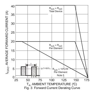
Notes: 5. Black Aluminium Heatsink; length 37mm, width 15mm, height 50mm.
