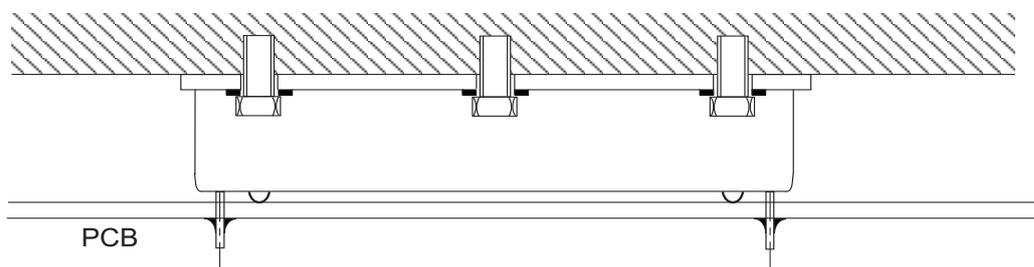
**Baseplate Case Fixing - Anti Vibration Mounting onto PCB**
