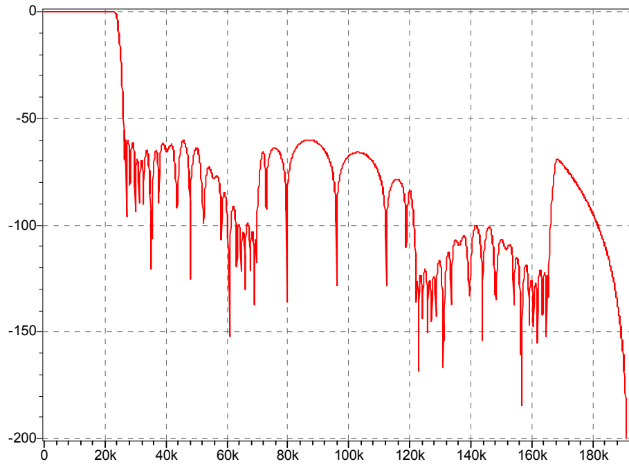
Figure 44 ADC Frequency Response up to 4 x fs. (Sample rate, fs = 48kHz)
