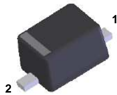
* Band Denotes Cathode SOD-323F
