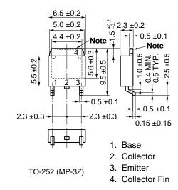
**Note** The depth of notch at the top of the fin is from 0 to 0.2 mm.
