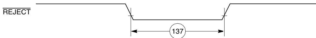
Figure 63. CAM Interface \overline{\text{REJECT}} Timing Diagram
