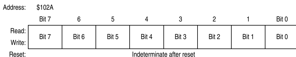
Figure 8-5. Serial Peripheral Data I/O Register (SPDR)
