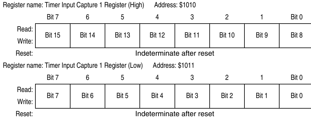
Figure 9-4. Timer Input Capture 1 Register Pair (TIC1)
