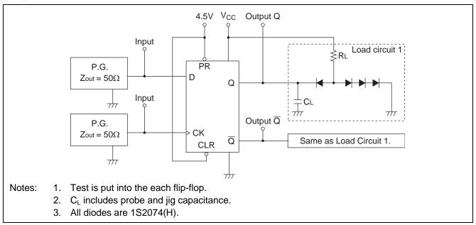
2.  $t_{PHL}$ ,  $t_{PLH}$  (Clear or Preset  $\rightarrow Q$ ,  $\overline{Q}$ )
