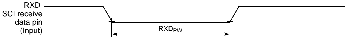
Figure 10-15 RXD Pulse Width
