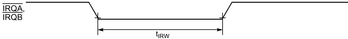
Figure 10-6 External Interrupt Timing (Negative-Edge Sensitive)
