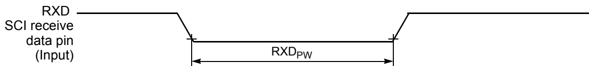
Figure 10-17 RXD Pulse Width
