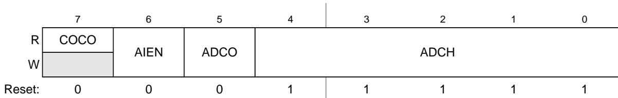
Figure 10-3. Status and Control Register (ADCSC1)
