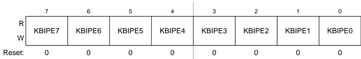
Figure 7-4. KBIx Pin Enable Register
