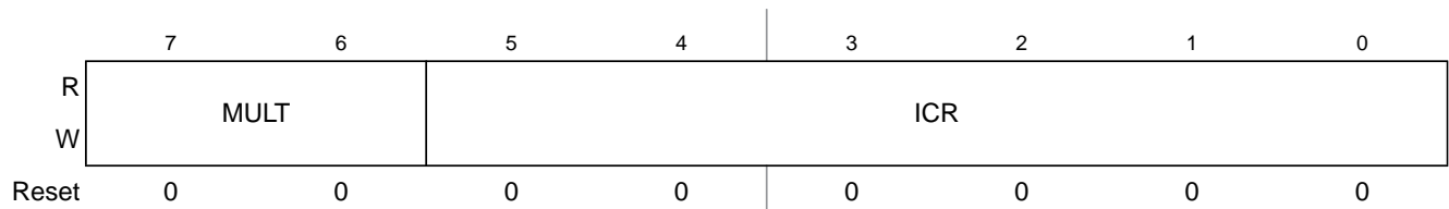
Figure 14-4. IIC Frequency Divider Register (IICF)
