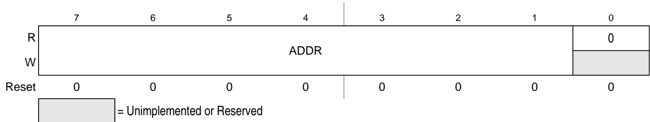
Figure 14-3. IIC Address Register (IICA)
