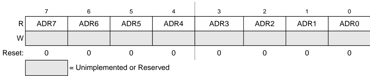
Figure 15-7. Data Result Low Register (ADCRL)
