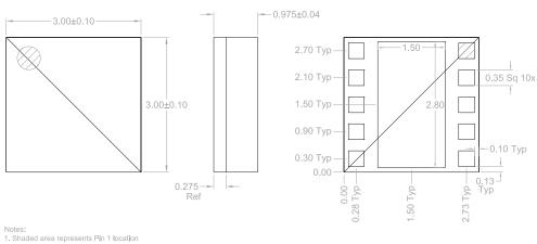
Defining VO Pad Center: To define center of the VO pad copring, draw a right triangle In one corner of the VO pad Then take the center of the hypotenuse to determine center of I/O pad
