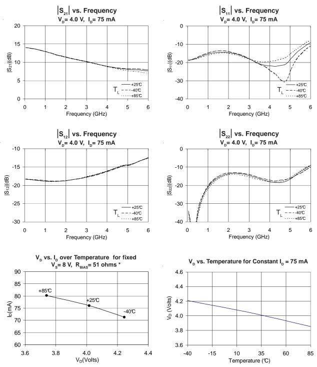
\* Note: In the applications circuit on page 4, R<sub>BIAS</sub> compensates for voltage and current variation over temperature.
