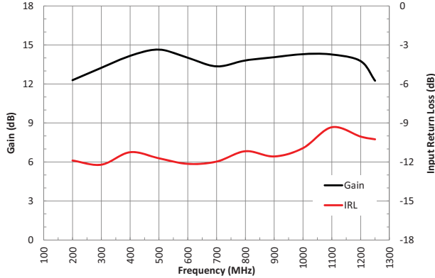
Gain/IRL versus Frequency, P OUT = 39.5dBm (CW, V_D = 28V, I_{DQ} = 88mA )
