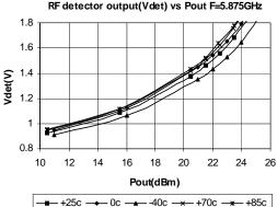
RF detector output(Vdet) vs Pout F=5.875GHz
