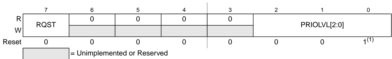
Figure 4-11. Interrupt Request Configuration Data Register 5 (INT_CFDATA5)
