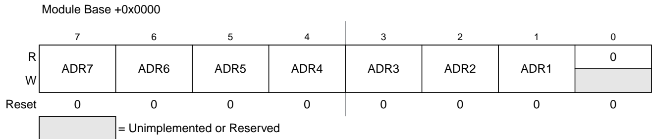
Figure 12-3. IIC Bus Address Register (IBAD)
