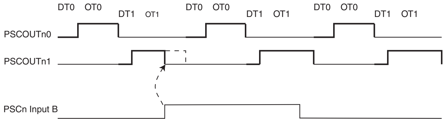
Figure 12-36. PSC behavior versus PSCn Input B in Mode 9.
