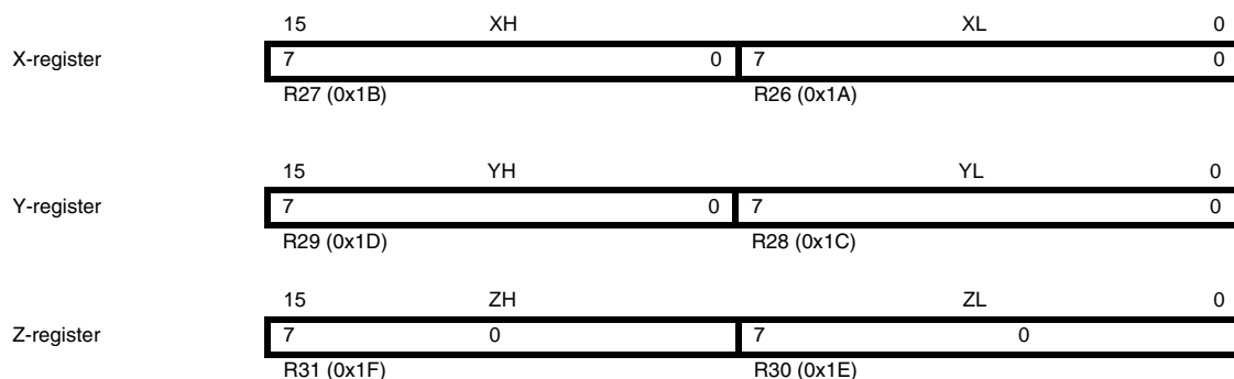
Figure 5-5. The X-, Y-, and Z-registers
