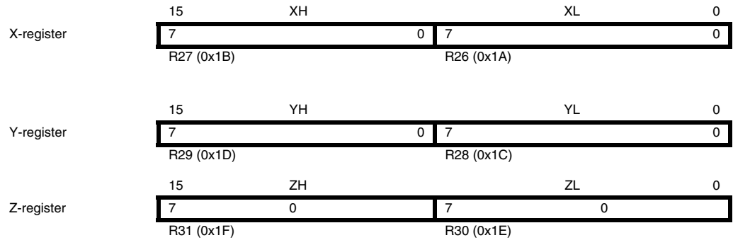
Figure 7-3. The X-, Y-, and Z-registers
