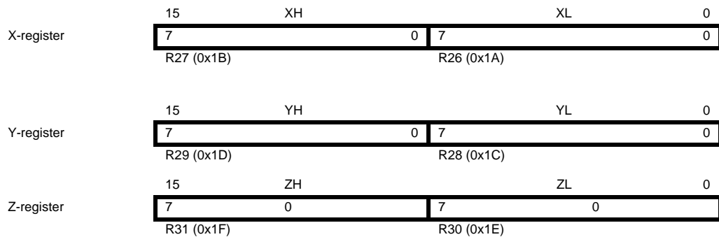
Figure 4-3. The X-, Y-, and Z-registers
