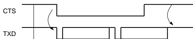
Figure 20-16. Transmitter Behavior when Operating with Hardware Handshaking
