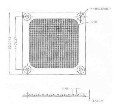
Aluminum/Stainless filters offer high levels of air passage while efficiently filtering contaminants and shielding EMI/RFI.
