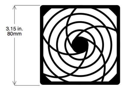
Material Plastic - reinforced ABS UL approved Rating UL94V-O
