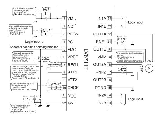
Each constant setting method for the above circuit diagram example is as follows : Current LIMIT (100%) set
