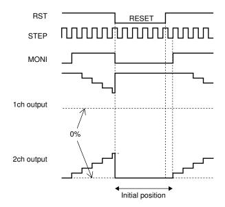
When the RST pin is set to Low, the excitation position of the output is forcibly set to the initial position, and the MONI output is placed in the ON state. When RST is then set to High, the excitation position is advanced by the next STEP input.
