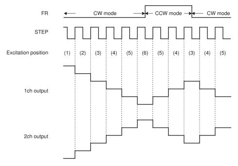
The internal D/A converter proceeds by one bit at the rising edge of the input STEP pulse.
