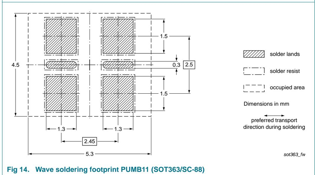
**Fig 14. Wave soldering footprint PUMB11 (SOT363/SC-88)**
